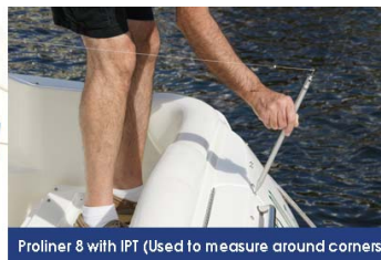
Proliner 8 with IPT (Used to measure around corners)
